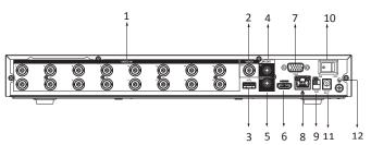
1 Video In 2 Video Out 3 USB Port 4 Audio In 5 Audio Out 6 HDMI Port 7 VGA Port 8 Network Port 9 RS-485 Port 10 Power Switch 11 DC 12V Power Input 12 Ground
